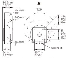
Holes are located to mount to a standard 4" square outlet box, or 2" wide gangable or non-gangable switch box.
